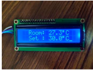
Fig. 12. LCD Display for Feedback
