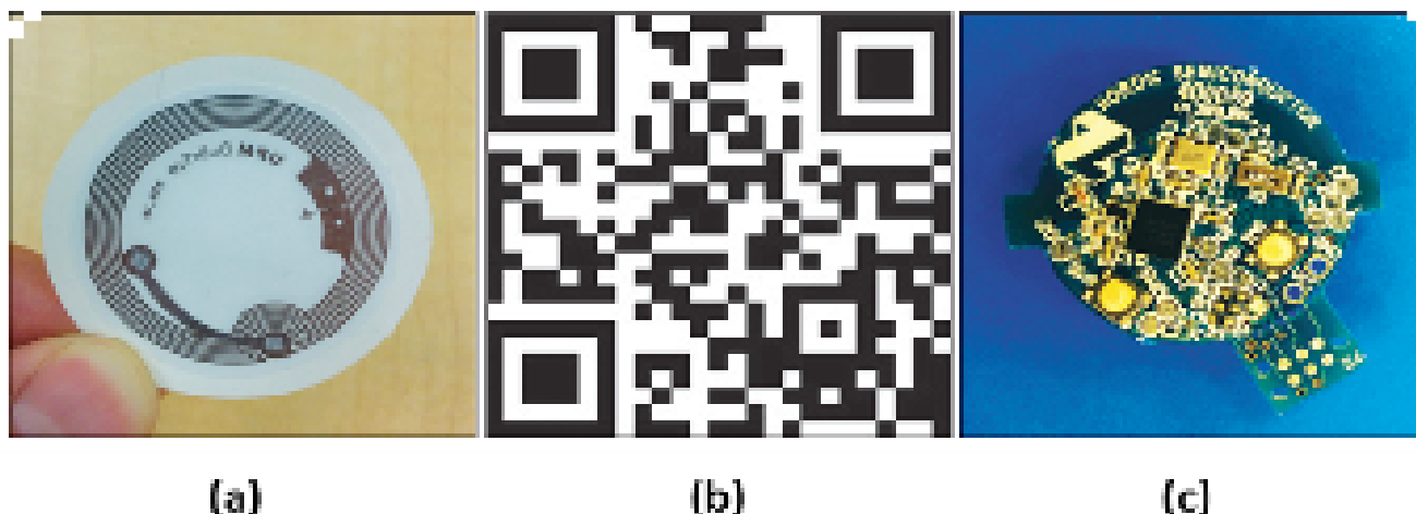
Fig. 3 : Tagging technologies for identification of IoT devices. (a) NFC, (b) QR code, (c) BLE tag
