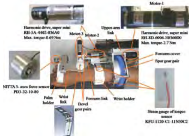
Figure 1: W-EXOS: 3DOF wrist and forearm motion assist exoskeleton robot
