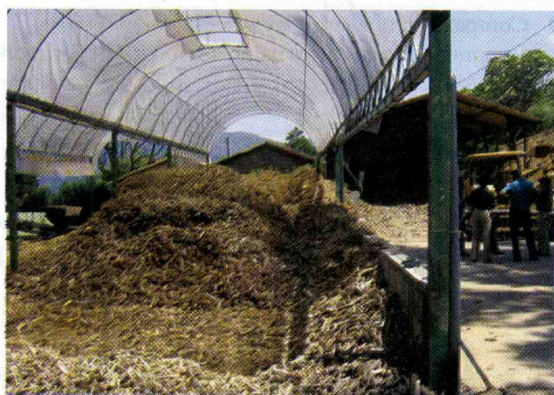
Fig 6. 1 MW Dendro power plant using fuelwood (Gliricidia) storage area
