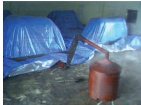
Figure 3: Smoke generated from paddy husk combustion within the stove conveyed to the stack
