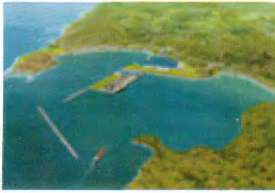
(i) Tsunami breakwaters/ Offshore breakwaters
