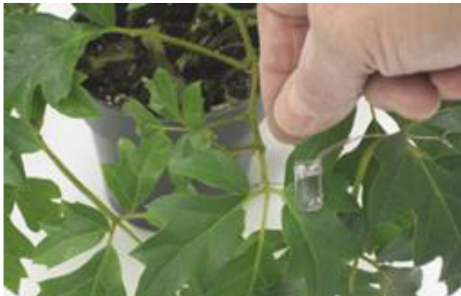
Fig.6 : Leaf thickness sensor developed for automated farming
