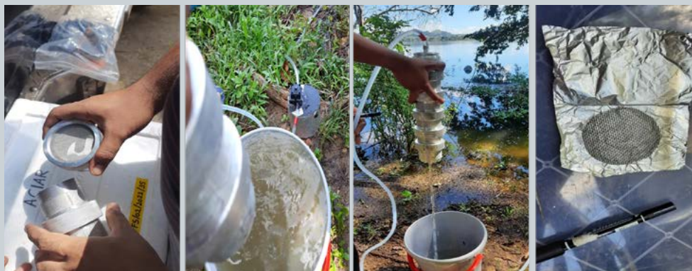
Figure 2.8.3: Sieving device used to sample water for microplastic analysis
