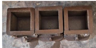
Fig. 1. Oil & grease applied (150×150×150mm) mould
