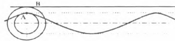
Fig.4 A trochoid curve is traced out by point A as the outer circle rolls along the base of line B [30]
